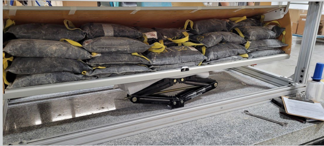
E175 bin Engineering inertial load test
