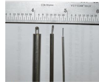
LEFT to RIGHT: 1/4" SS sheath TC; 1/8" SS sheath TC; 1/16" SS sheath TC
